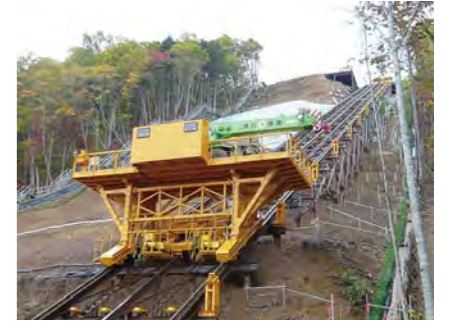
Inclined equipment with a maximum 30 t capacity, for steep terrain.
