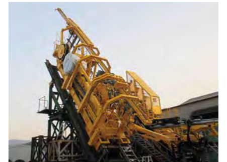
Jumbo inclined-shaft cart equipment for a 50° rail slope.
